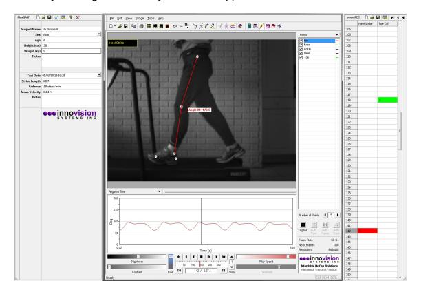
System Includes: MaxGAIT 2D software, 60/120Hz camera, IR Light and Markers
