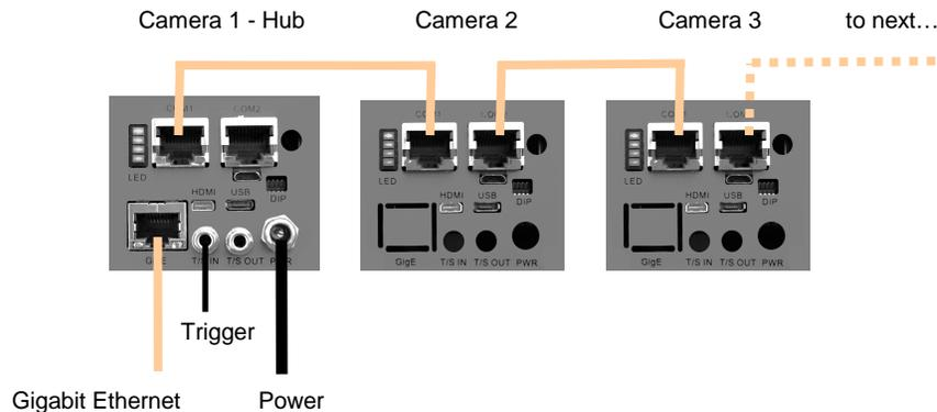
Use IP address in the range 169.254.x.x. This is the default assigned by Windows. However, we recommend setting the IP address manually to 169.254.21.1 with Subnet mask 255.255.255.0.
